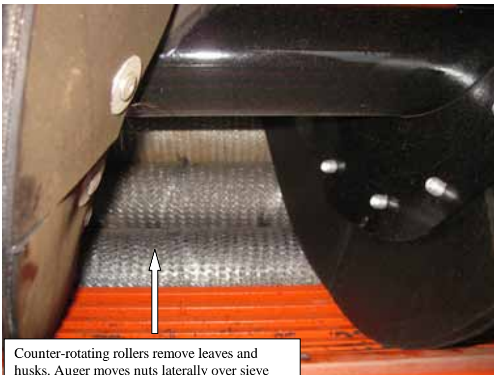
Front mounted Jolly pick-up harvester, with side sweeper
