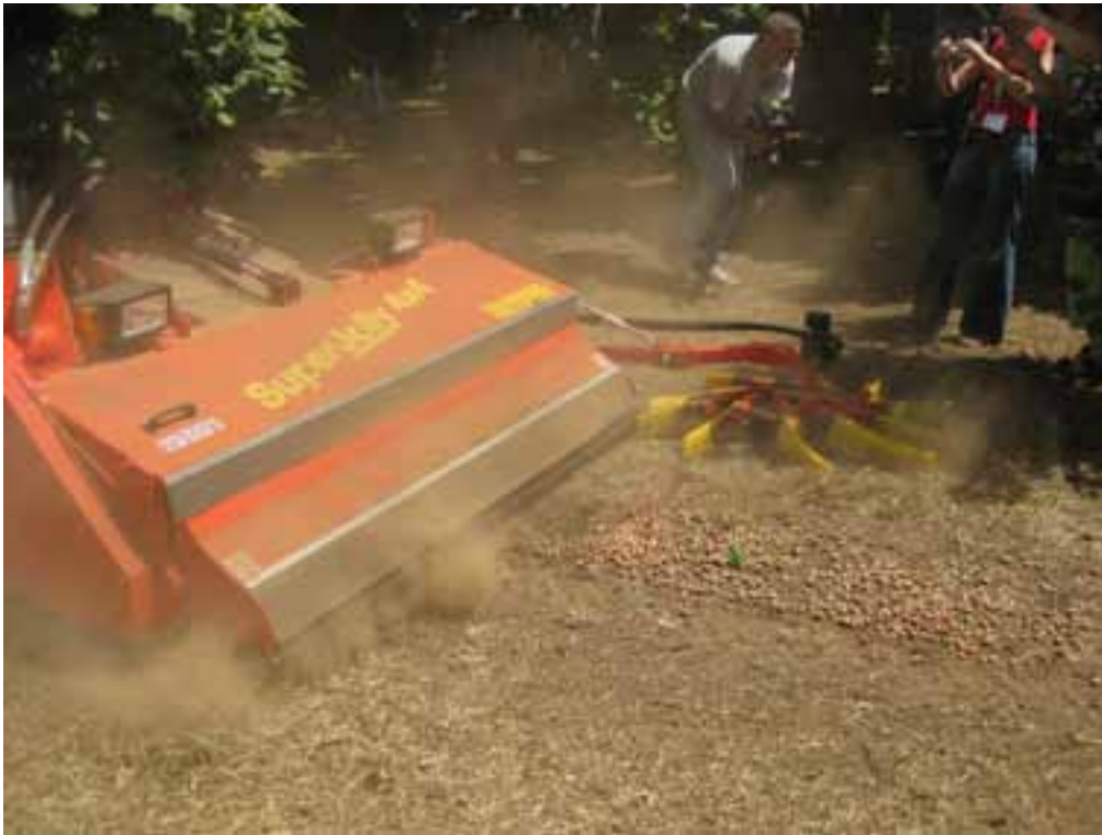
Front mounted Jolly pick-up harvester, with side sweeper
